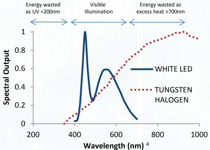
~75% of output from tungsten halogen lamps is wasted as heat and UV compared to LED sources.
