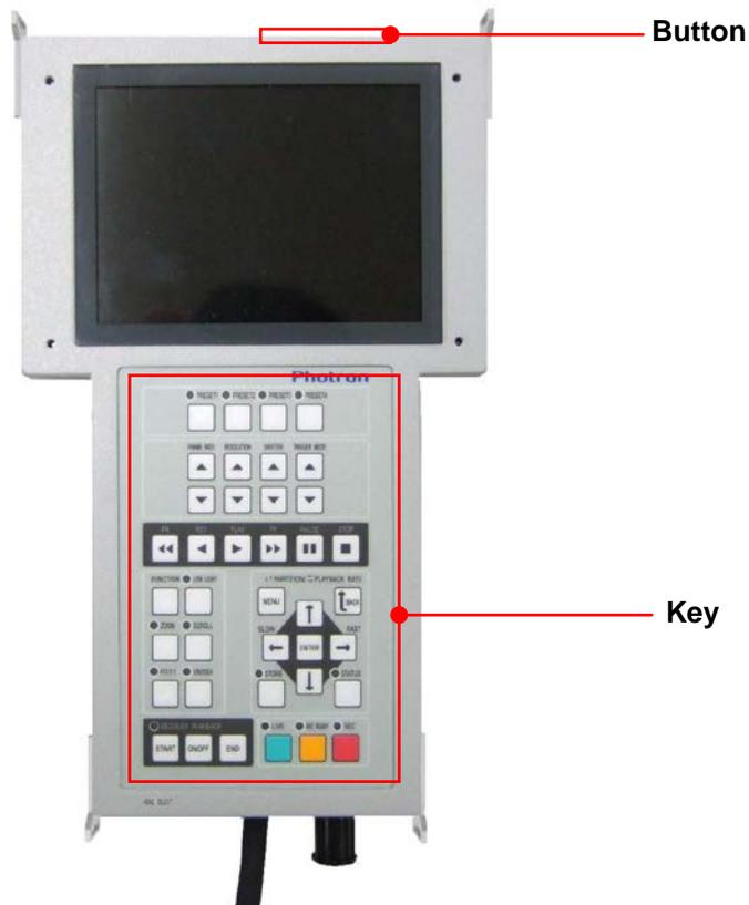
■ Keys (on the Keypad front panel)
