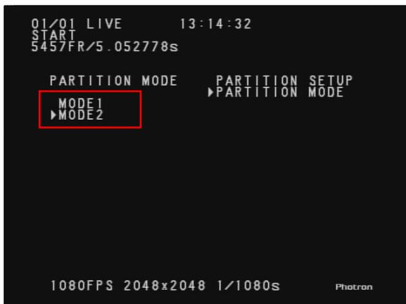
[MODE1]: "Recording to a partitioned section" operation as previously explained (p. 39).
