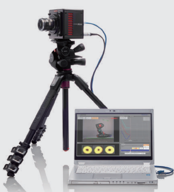
Phoo Schlieren imaging of fuel injection and engine combustion 20,000fps
