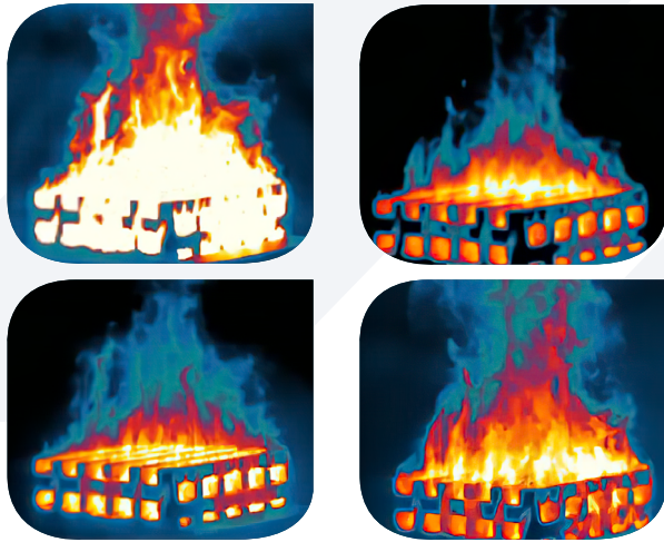
Multispectral image of burning wood crib
