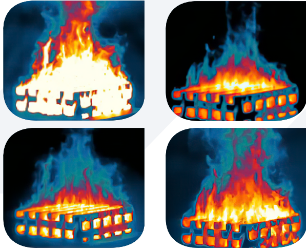
Multispectral image of burning wood crib
