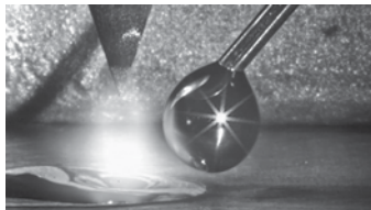
TIG WELDING - (LABSOLDA, CAVILUX HF)
