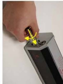
7. Connect laser cable
