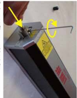
2. Insert fiber and lock it
