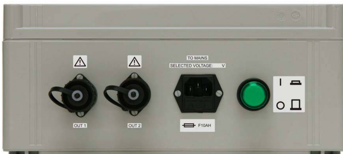
Fig. 3.9. Front view of laser unit power supply.
