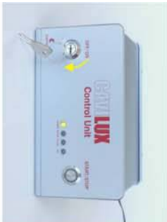
16. Switch on control unit
