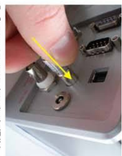
5. Connect remote interlock (RIL)
