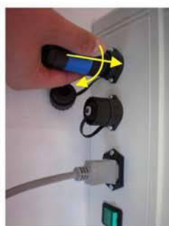
10. Connect laser power cable
