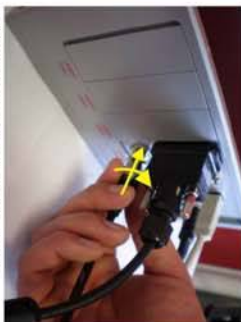
13. Connect camera trig cable
