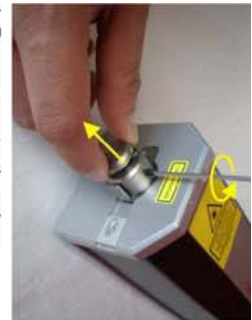
1. Remove protection plug
