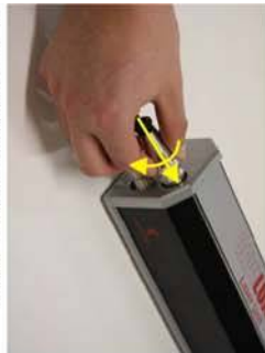
11. Connect laser power cable
