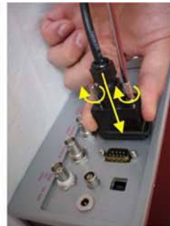
6. Connect laser cable
