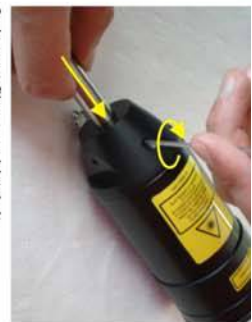
3. Insert fiber and lock it
