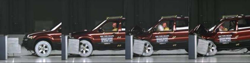
Photron's high-speed camera captures a 40 mile per hour vehicle impact test. All vehicles are subjected to rigorous crash and sled tests, every one of which must be recorded at 1,000 frames per second for the engineers to analyze to see how the vehicle and dummy occupants interact. These images are selected from the original 1,000 fps recording.
