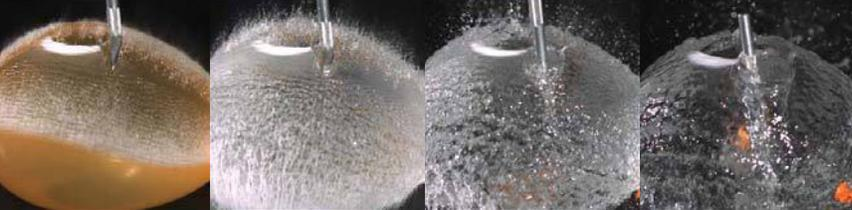
Photron's super sensitive high-speed camera records a scalpel puncturing a water filled balloon. These images are a selection from the original sequence recorded at 4,000 frames per second with a 25 microsecond shutter. The images clearly show the balloon tearing while the water retains the original balloon shape even after the scalpel has passed right through it.
