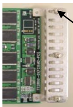
Guide Plate and its retaining screws
